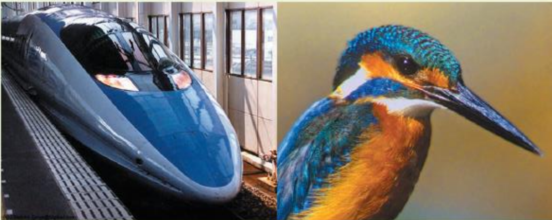
The design features of Japan's Shinkansen 500-Series exemplifies biomimicry in action. Its overhead pantograph sports serrations were modeled on the design of owl plumage to reduce air resistance noise, and the air piercing nose cone design was inspired by the kingfisher's beak. Photo: Steve Auer/Associated Press; owl: iStockphoto
